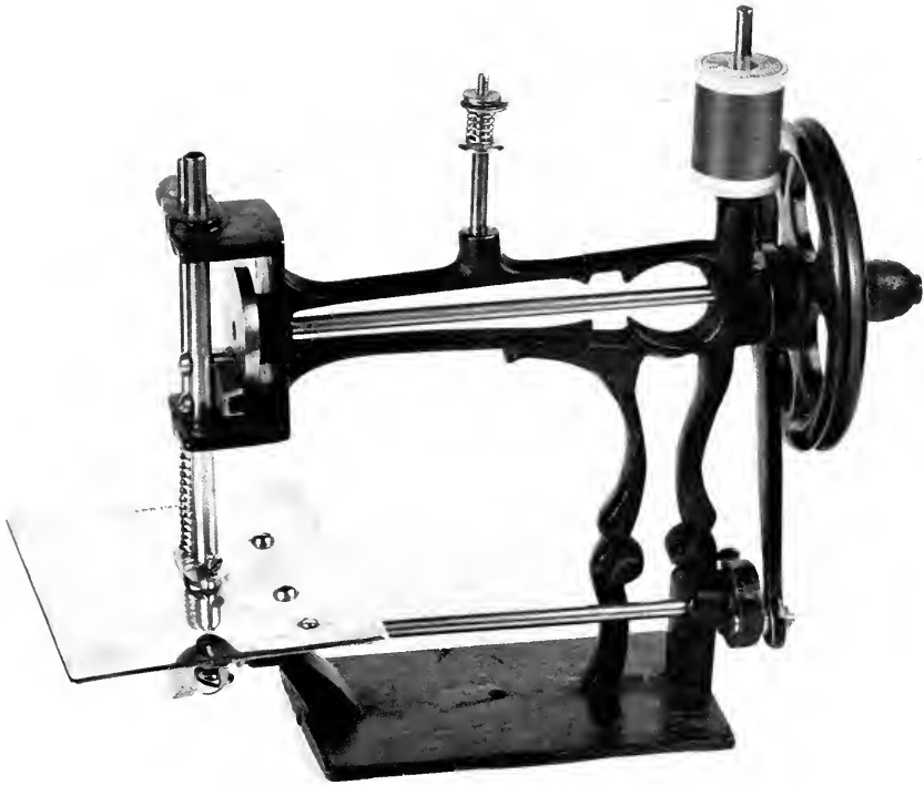
Figure 71.—ATLANTIC SEWING MACHINE, 1869. This machine is typical of the many varieties manufactured for a very short time in the 1860s and 1870s. It is about the size of the average hand-turned variety, 8 by 10 inches, but lighter in weight. The frame design was the patent of L. Porter, May 11, 1869, and the mechanism was patented by Alonzo
